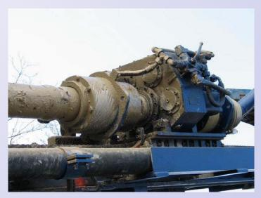
Based on success in other types of heavy equipment, a customer approached Kalsi Engineering in 2006 to provide rotary seals for the air/water swivel in newly designed reverse circulation drilling machine. After several years of experience, the customer reported 1,800 hours of sealing life with Kalsi Seals, compared to less than 150 hours with conventional greased seal assemblies.
