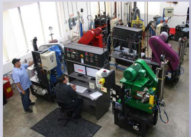
*Kalsi Engineering performs an average of 10,000 hours of rotary seal testing every year. Much of the testing is aimed at developing seals capable of surviving higher temperatures at higher pressures and speeds for longer durations.*
