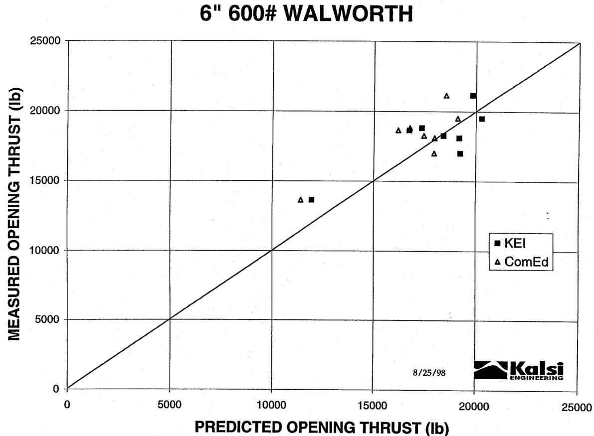
Note: Valve stiffnesses obtained from closed-form equations.
