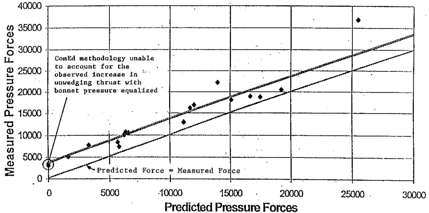
Figure 1. ComEd Methodology Prediction vs. Measured Portion of Unseating Thrust Due to Pressure Locking Forces for the Borg-Warner Valve Tested by ComEd [1]
