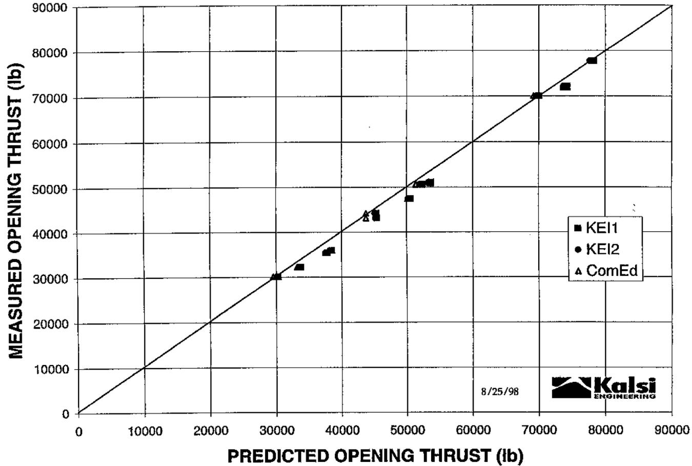
Note: For KEI1, valve stiffnesses obtained from FEA; for KEI2, valve stiffnesses obtained from closed-form equations.
