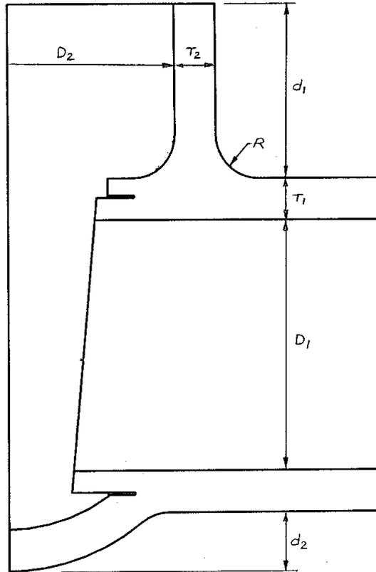
**Figure 5(c). Key Body Dimensions Used in the Three-Dimensional Finite Element Model for Valve Body Flexibility Analysis**
