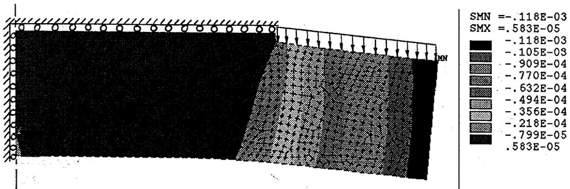
Figure 4. Finite Element Model for ComEd 10", Class 300 Borg-Warner Valve Disc Including Hub Flexibility for Disc Flexibility Analysis
