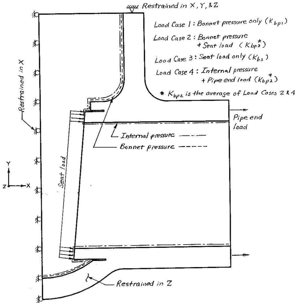
**Figure 5(b). Load Cases and Boundary Conditions Used in the Three-Dimensional Finite Element Model for Valve Body Flexibility Analysis**
