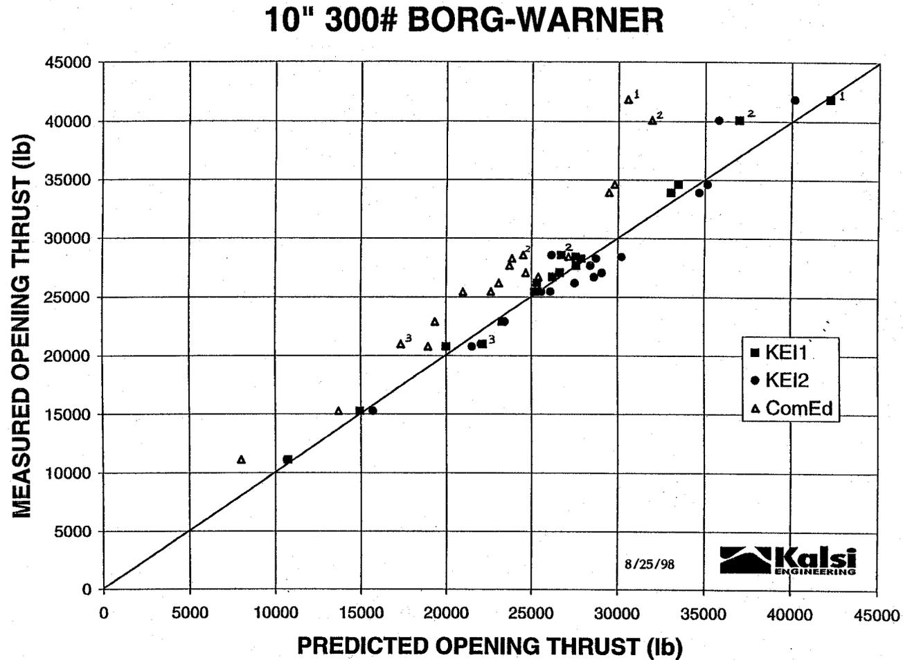
Figure 6. Comparison of KEI Generalized Methodology and ComEd Methodology Pressure Locking Predictions vs. Unwedging Thrust Test Results for the 10" Class 300 Borg-Warner Valve
