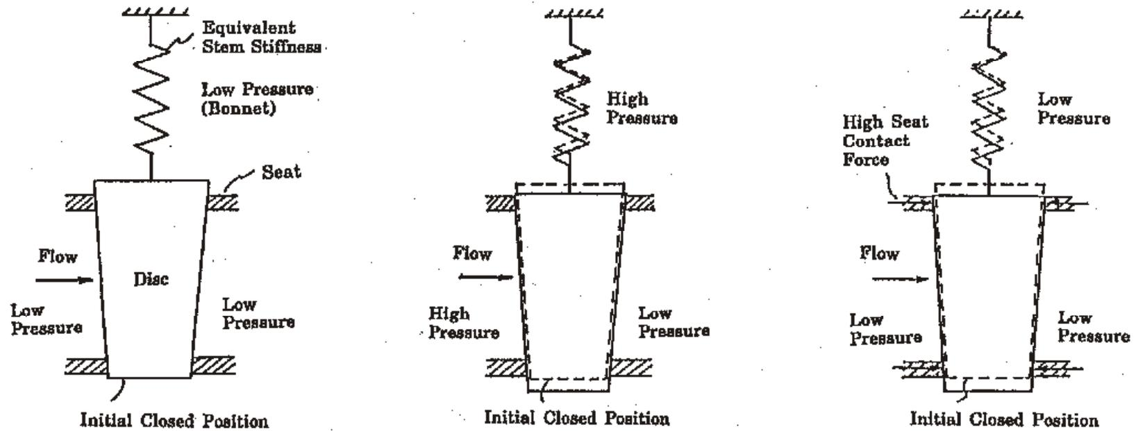
Figure 2. Disc Pinching Phenomenon Caused by the Combination of Body Flexibility and a Sequence of Upstream Pressure Changes between Valve Closing and Opening
