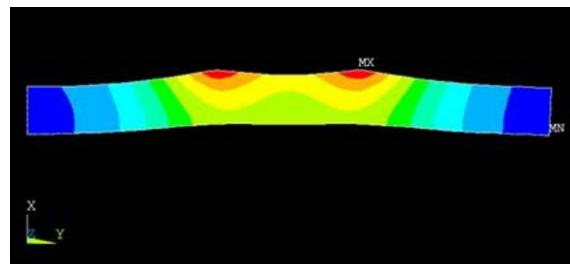
**Figure 2****Use FEA to estimate shaft thermal expansion**
