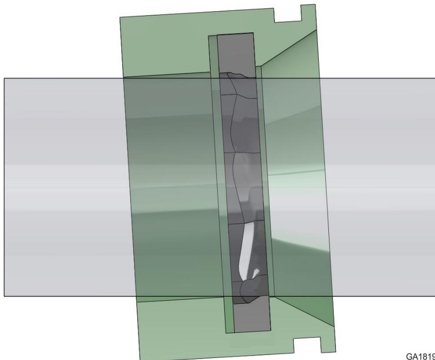
**Figure 4****Short bearing length can cause undesirable seal skew**
