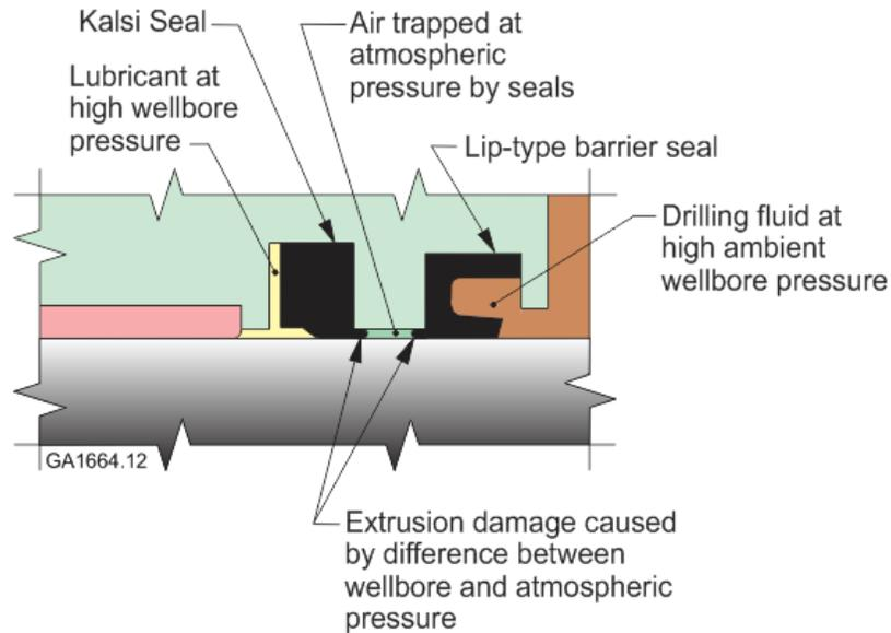
(b) Rotary seals are damaged by difference between wellbore and trapped atmospheric pressures
