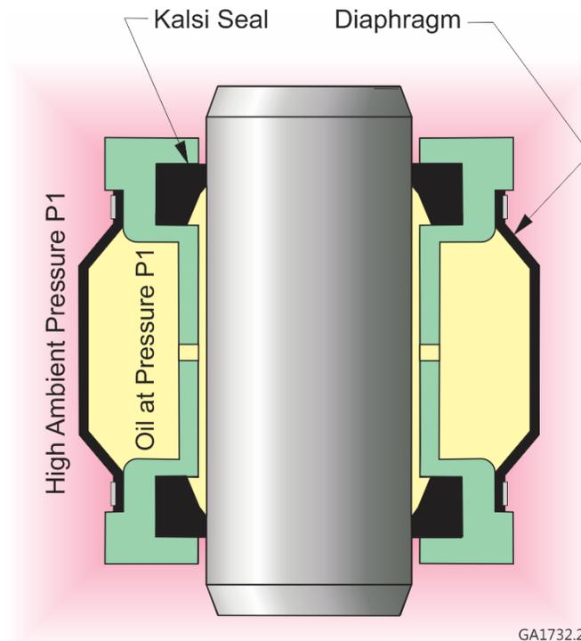
**Figure 5****Schematic of a diaphragm for preventing pressure locking**
