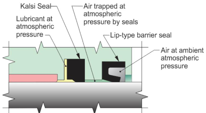
(a) Air trapped between rotary seals at time of assembly
