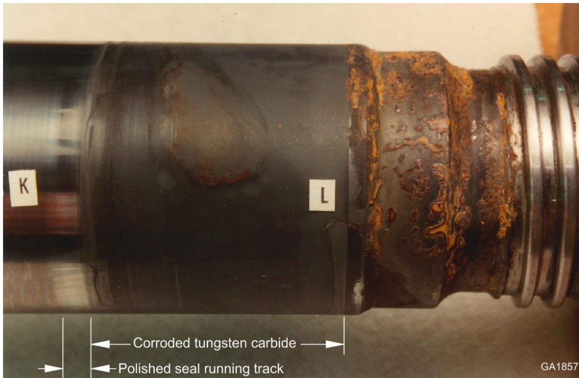
Figure 7 Corroded cobalt-based tungsten carbide coated sealing surface
