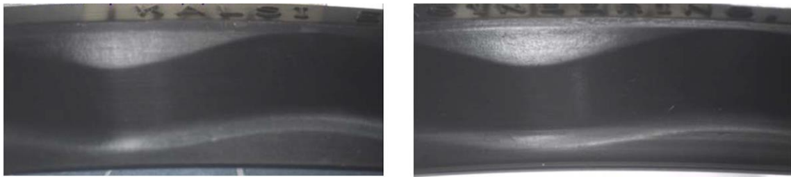
Figure 4 Before (left) and after (right) of the mud side seal from Test #2
