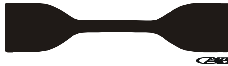
Figure 1 Typical Elastomer Tensile Test Coupon
