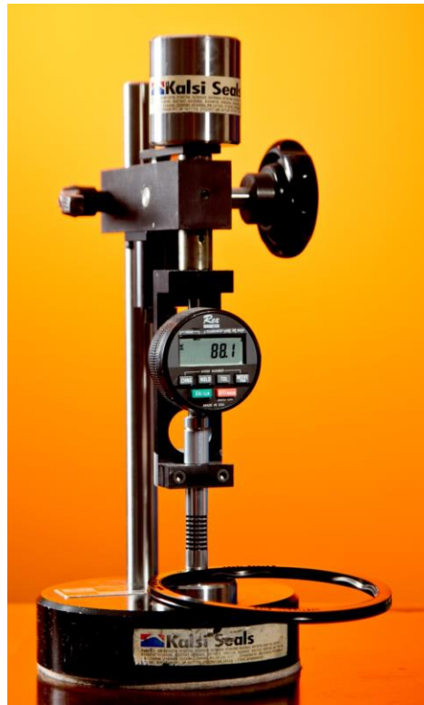
Figure 5 Example of Durometer gauge with stand
