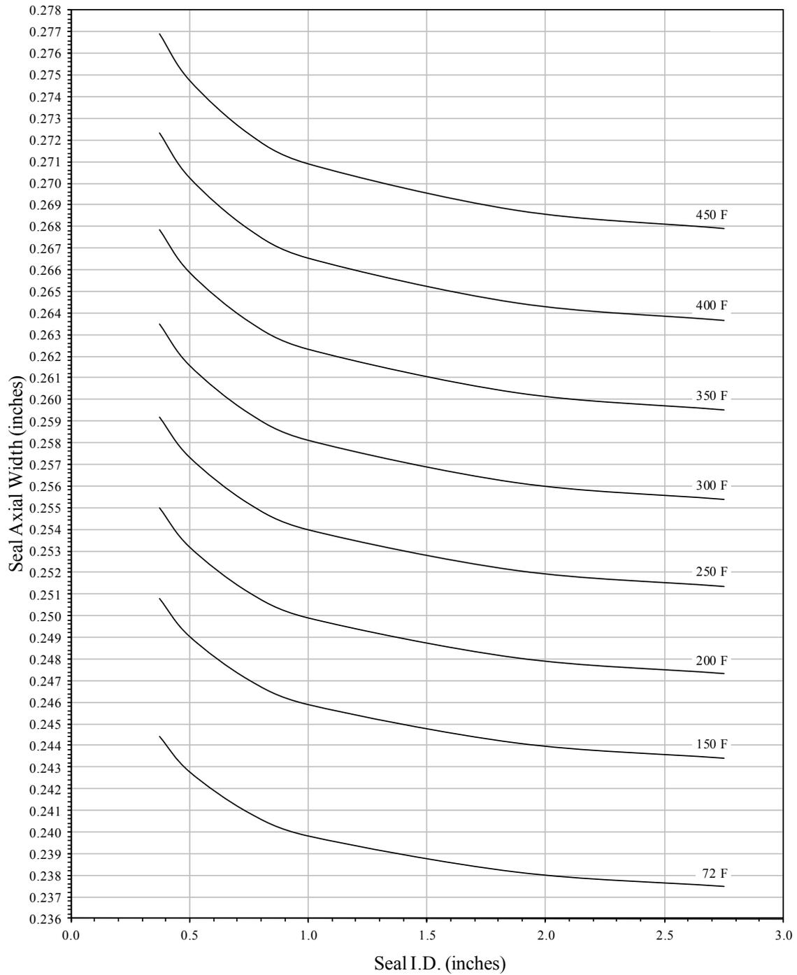
Axial Widths of **MMC 0.212" X 0.220"** Cross Section
