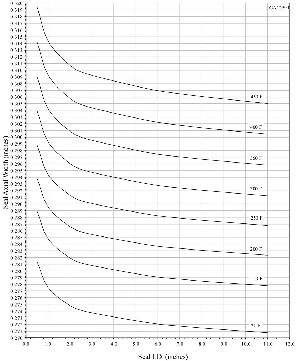
Axial Widths of **Nominal 0.415" X 0.300"** Cross Section
