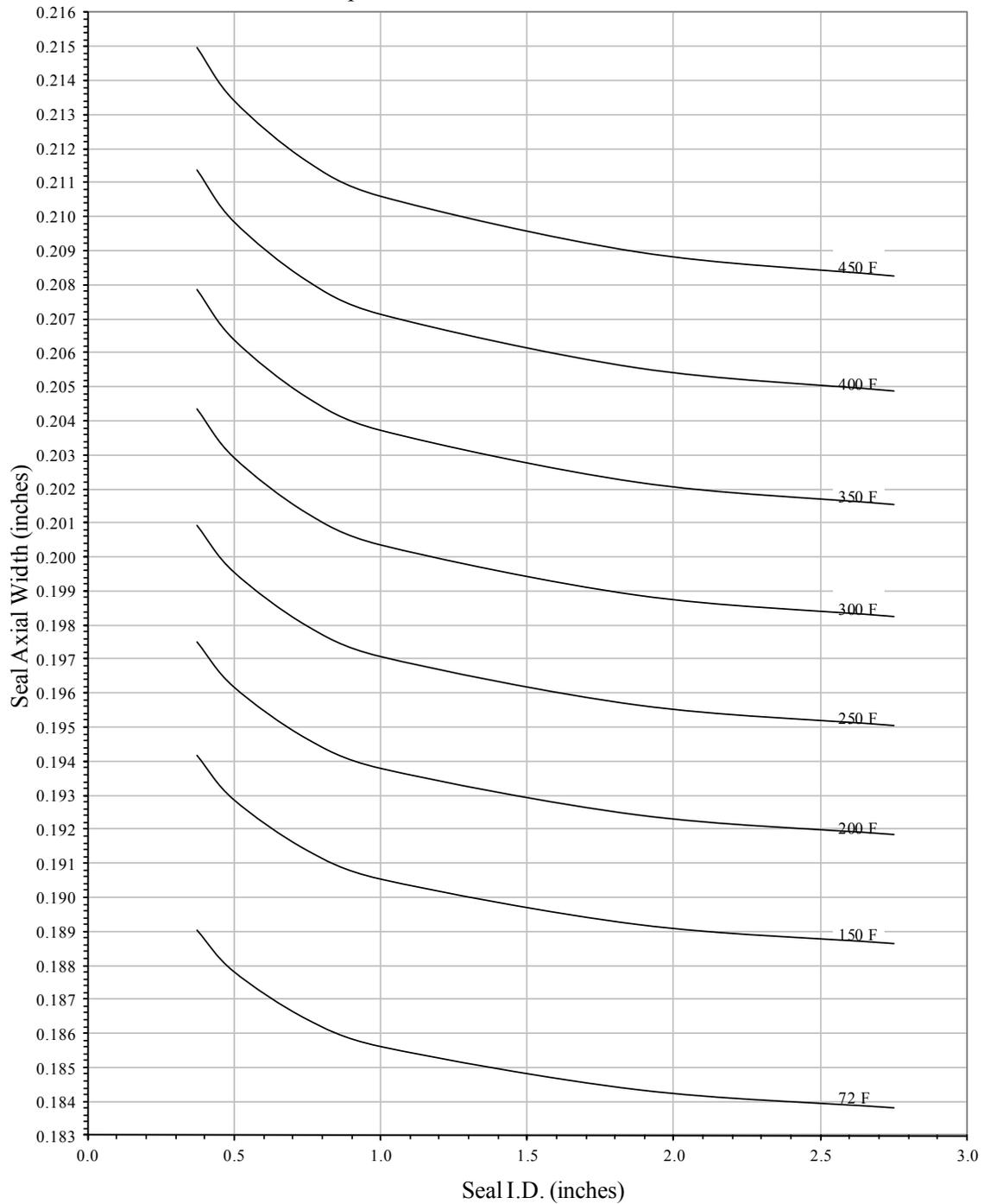
Axial Widths of **MMC 0.186" X 0.170"** Cross Section
