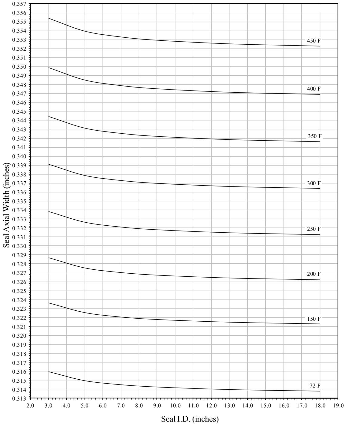
Axial Widths of **MMC 0.415" X 0.300"** Cross Section
