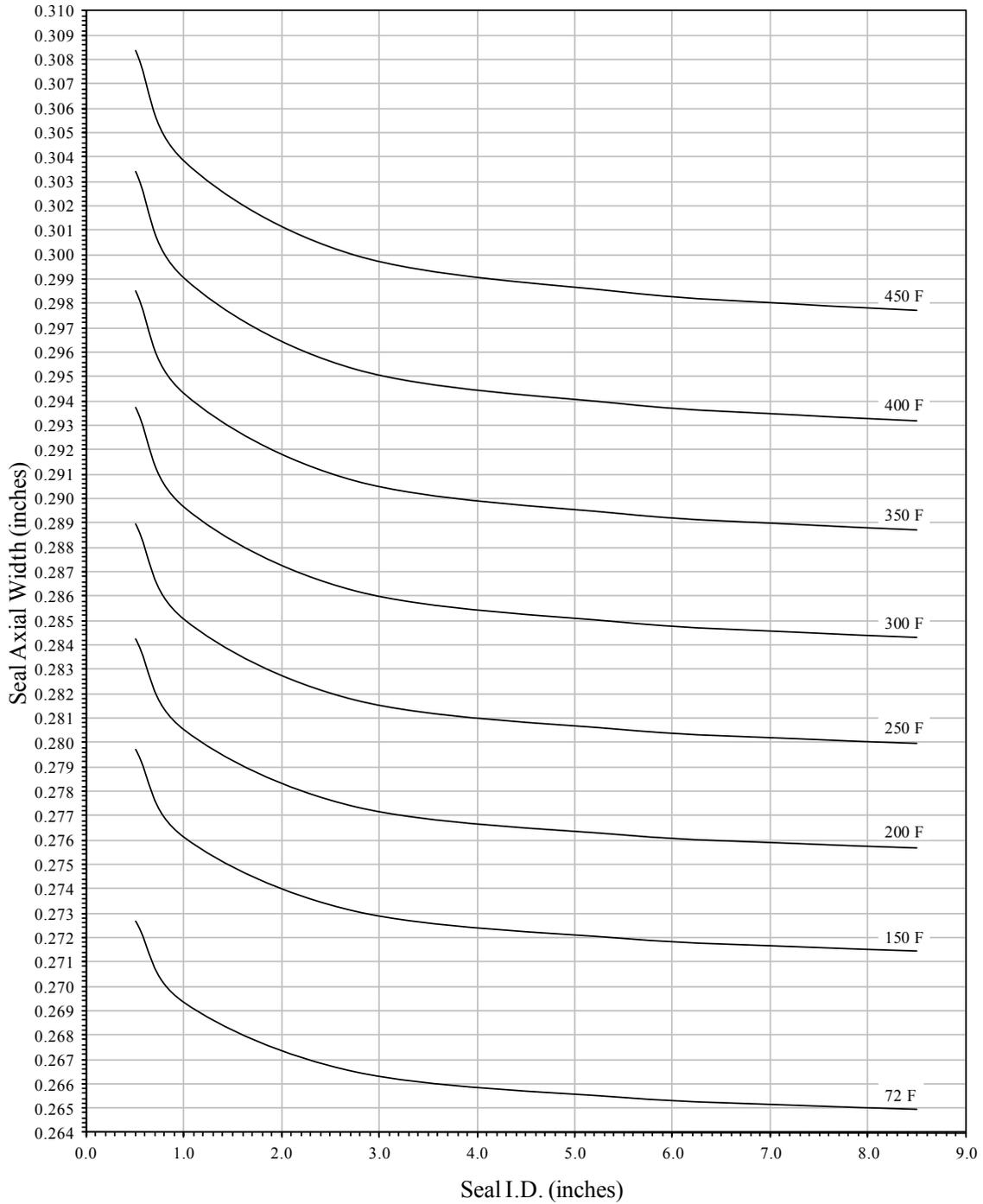
Axial Widths of MMC 0.270" X 0.250" Cross Section
