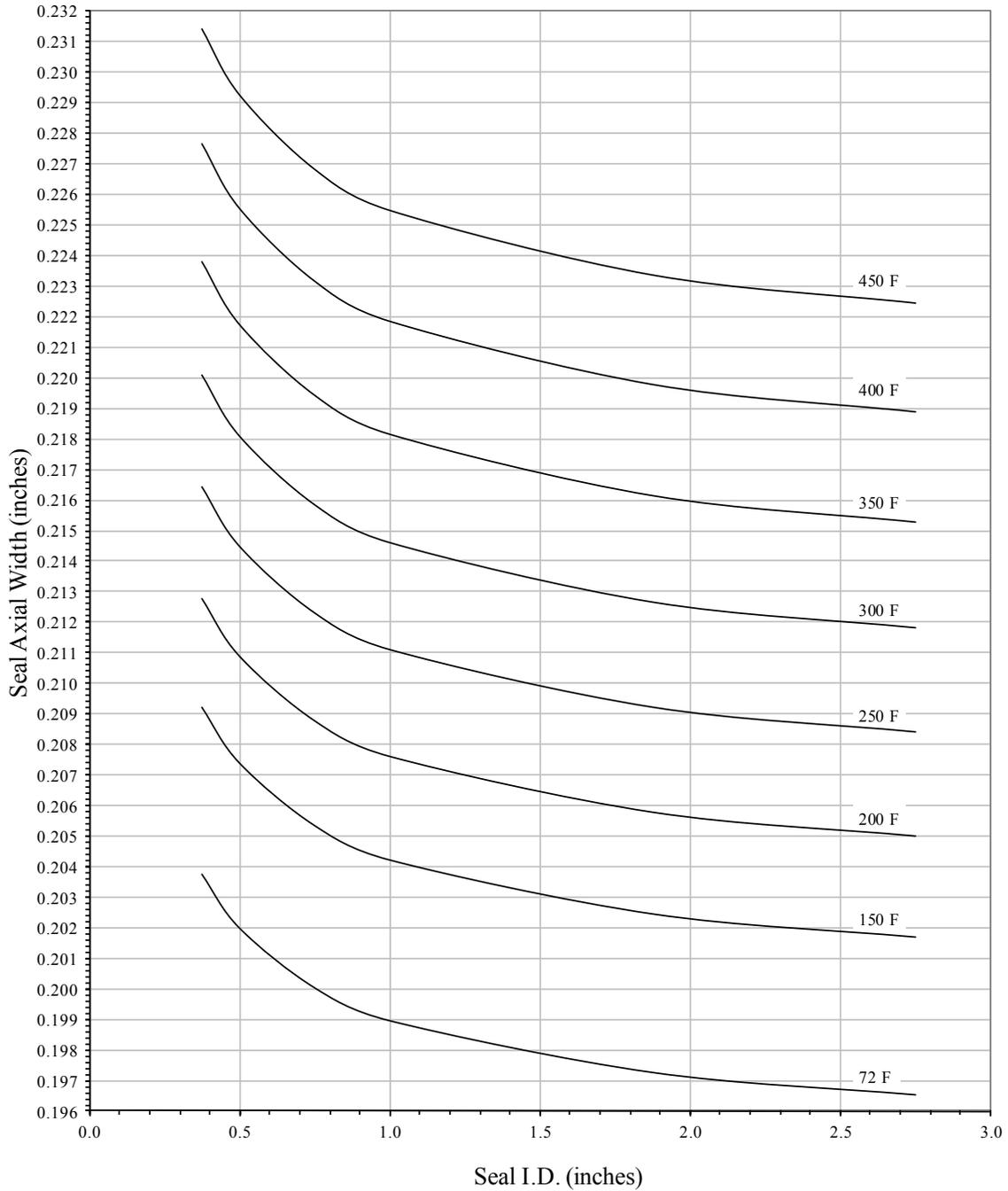
Axial Widths of **Nominal 0.186" X 0.170" Cross Section**
