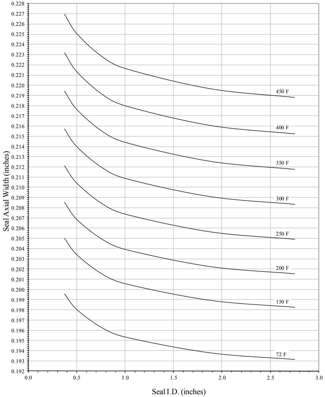
Axial Widths of **Nominal 0.212" X 0.220"** Cross Section
