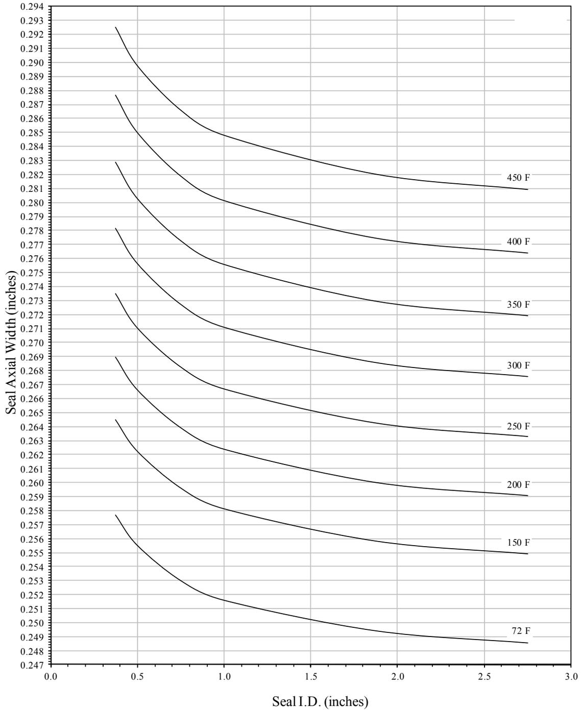
Axial Widths of **Nominal 0.270" X 0.250" Cross Section**
