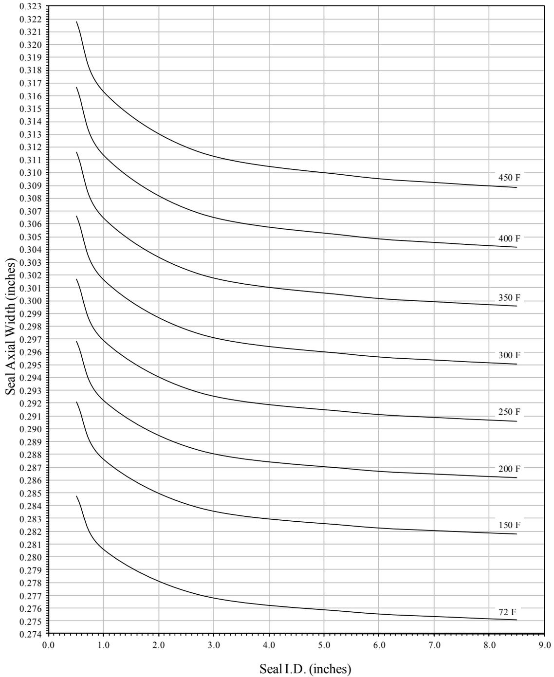
Axial Widths of **Nominal 0.335" X 0.25"** Cross Section
