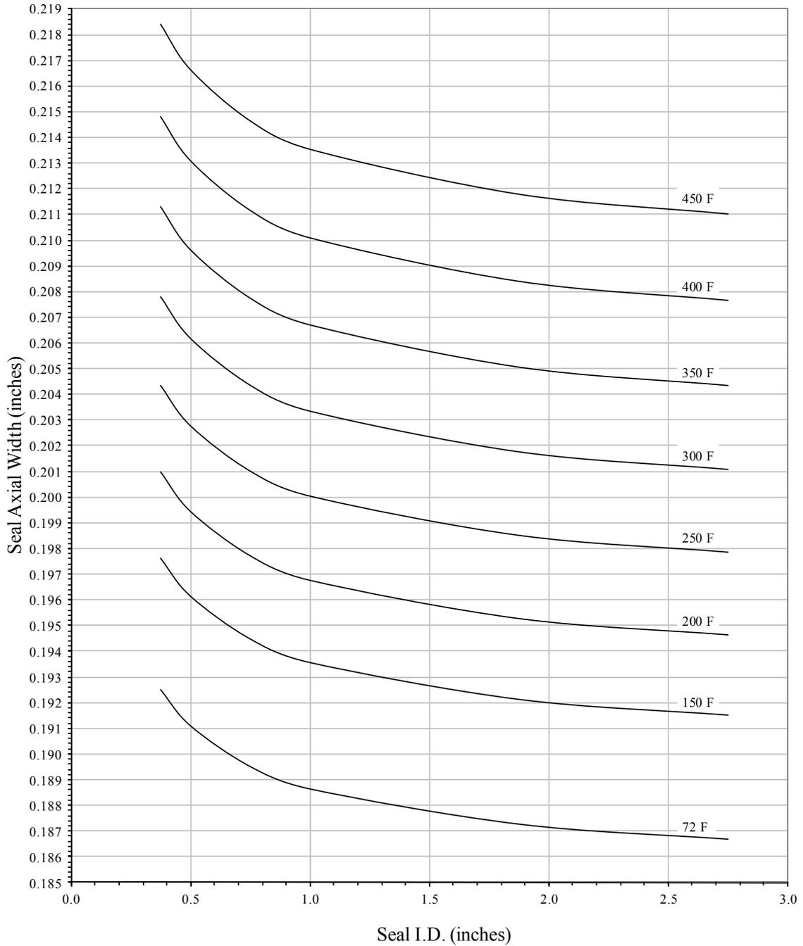
"Axial Widths of MMC 0.145" X 0.170" Cross Section
