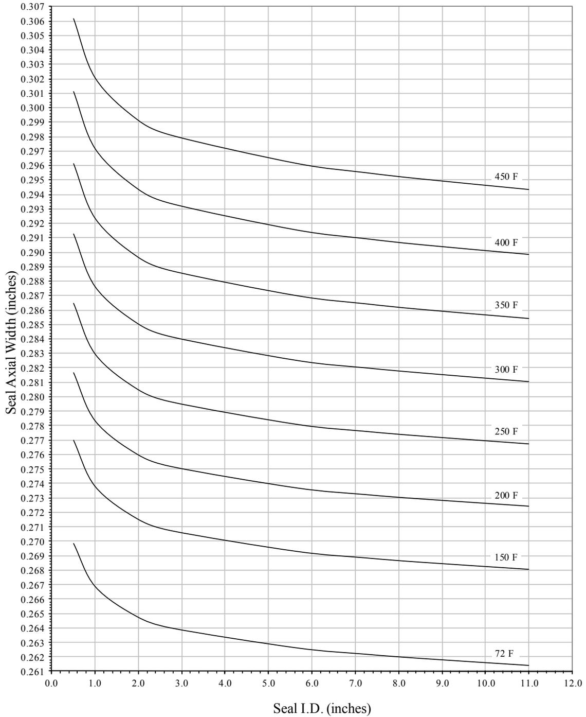
Axial Widths of **MMC 0.335" X 0.25"** Cross Section
