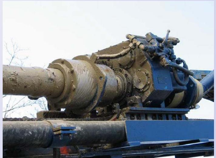
*Based on success in other types of heavy equipment, a customer approached Kalsi Engineering in 2006 to provide rotary seals for the air/water swivel in newly designed reverse circulation drilling machine. After several years of experience, the customer reported 1,800 hours of sealing life with Kalsi Seals, compared to less than 150 hours with conventional greased seal assemblies.*
