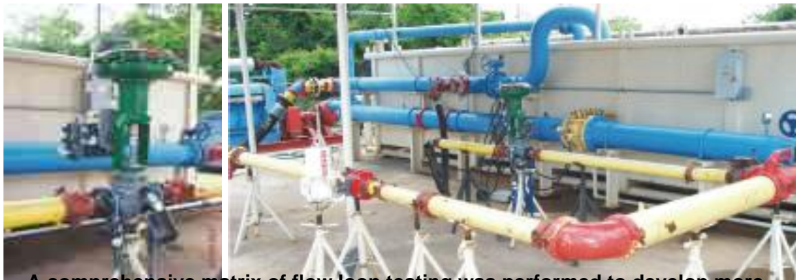
A comprehensive matrix of flow loop testing was performed to develop more accurate validated models for AOVs incorporated in KVAP.
